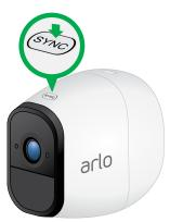
The LED on the camera LED lights blue and blinks rapidly to confirm syncing.
