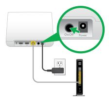
The Power LED and Internet LED on the front of the base station light green in about two minutes.
